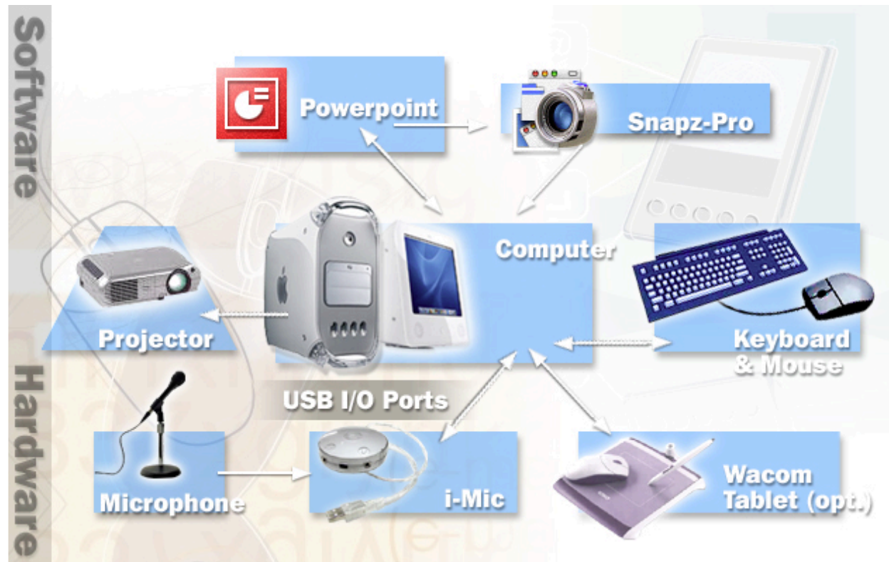
Figure 1. Hardware and Software Diagram for Recording Lectures
